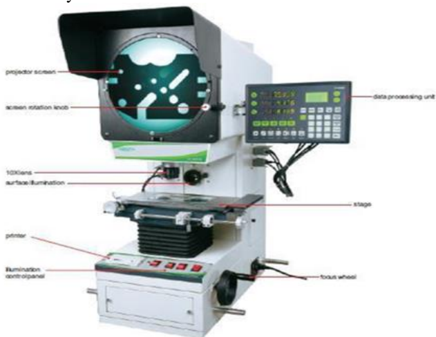
Fig.2- Profile Projector Machine
