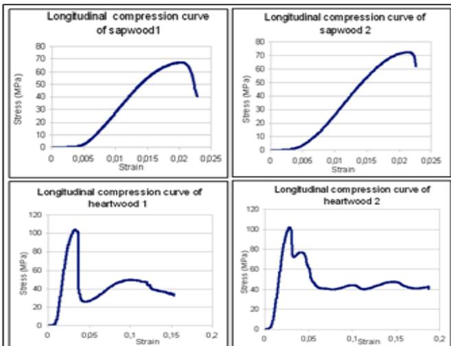
Figure.1: stress-strain curves in longitudinal compression of two specimens of sapwood and heartwood.
