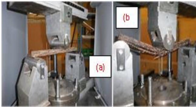
Image.2: Specimen in bending 3 points: (a) unloaded specimen; (b) specimen ruptured.
