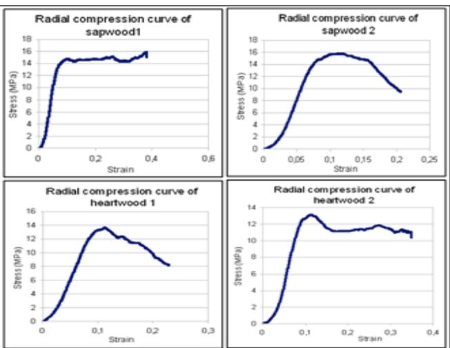
Figure.2: stress-strain curves in radial compression of two specimens of sapwood and heartwood.
