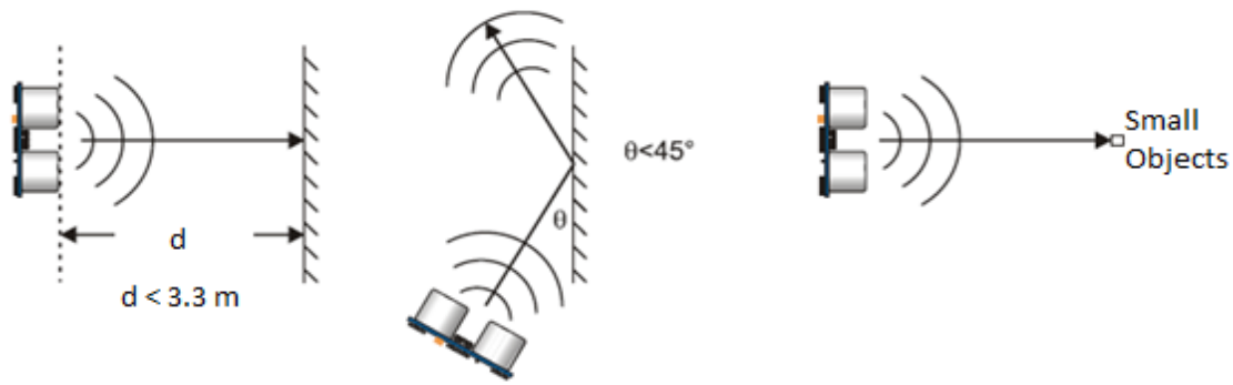
Fig.2.3: The application conditions of ultrasonic receiver – transmitter pair [6].
