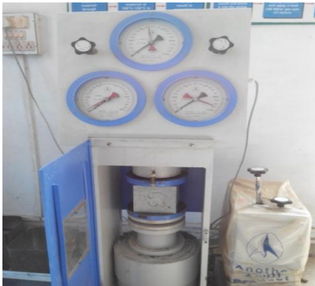
Fig. 4. Compressive Strength Testing Machine
