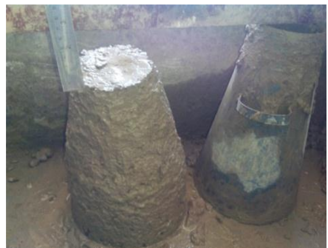
Fig. 3. Measurement of Slump
