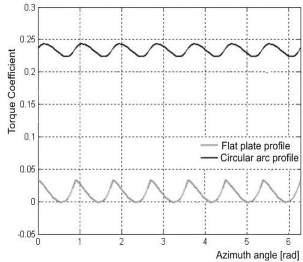
Fig. 10 Variation of the torque coefficient with the azimuth angle for the cases of flat plate and circular arc rotors with seven blades.
