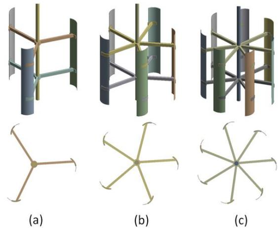
Fig.7 Rotors with different number of circular arc blades.
