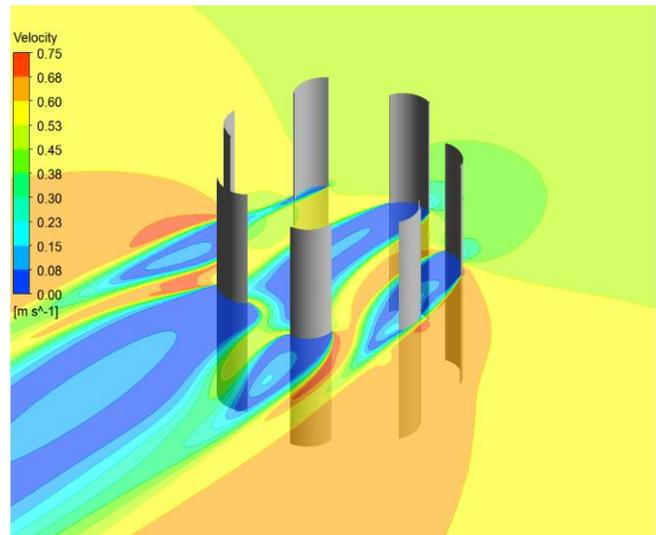
Fig.13 Dynamic simulation of the flow field around a rotating rotor with seven circular arc blades.
