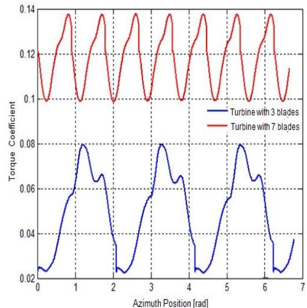
Fig.14 Dynamic simulation of two rotors with three and seven circular arc blades.
