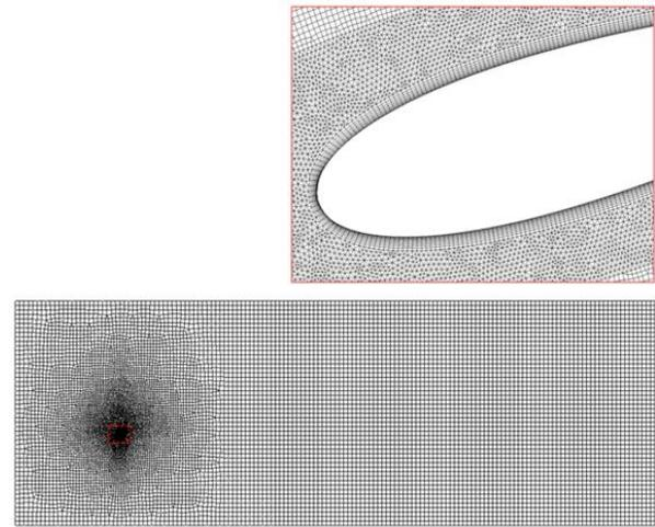
Fig.3 The computational mesh used to discretize the fluid domain.
