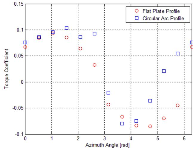
Fig.6 Torque coefficient obtained from a single blade simulation in different azimuth angles for the flat plate and circular arc profiles.
