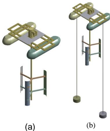
Fig.16 Two possible installation arrangements for hydrokinetic turbines.
