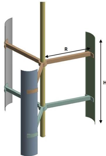
Fig. 1 Vertical axis hydrokinetic rotor with three blades.
