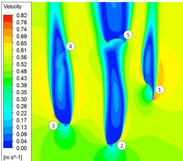
Fig.12 Static simulation flow field of a rotor with five blades.
