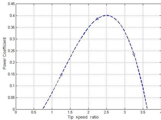
Fig.15 Variation of the predicted Power Coefficient of a hydrokinetic turbine as function of the tip speed ratio.
