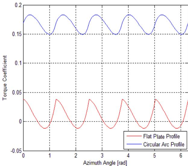
Fig.9 Variation of the torque coefficient with the azimuth angle for the cases of flat plate and circular arc rotors with five blades.
