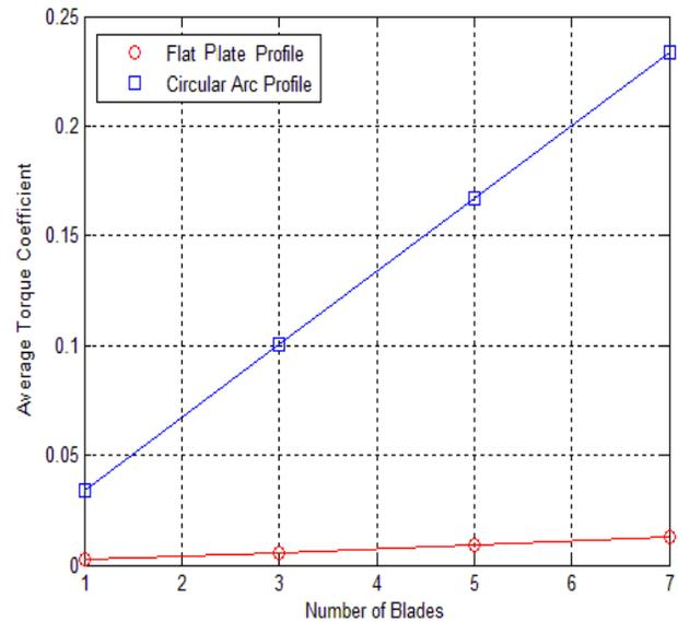
Fig.11 Comparison of the average torque coefficient produced by the flat plate and circular arc profiles rotors.
