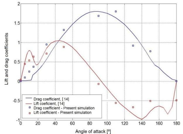
Fig.4 Simulations of NACA 0018 profile and the results were compared with the results of Sheldahl and Klimas [19].
