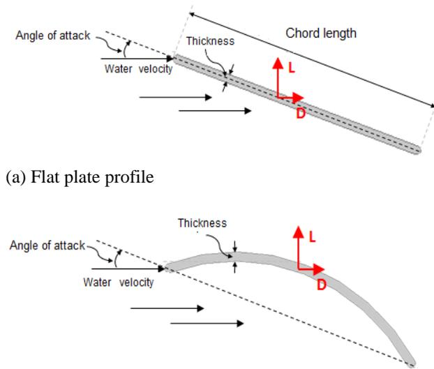
Fig.2 Investigated profiles, a) Flat plate profile, b) Circular arc profile.
