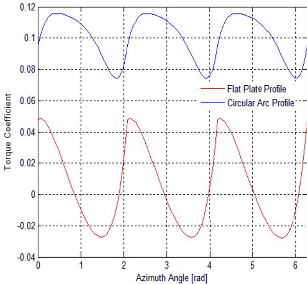
Fig.8 Variation of the torque coefficient with the variation of the azimuth angle for the cases of flat plate and circular arc rotors with three blades.
