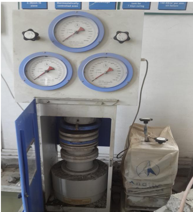
Figure - A set-up of Compression testing machine (CTM)
