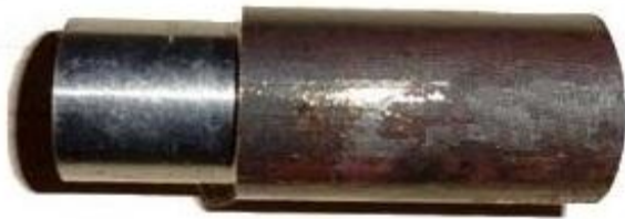
Fig. 2. Turned EN-18 Workpiece
