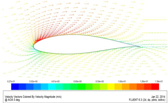
Fig22: Velocity vectors colored by velocity magnitude at 5° AOA with the SST k- $\omega$  model
