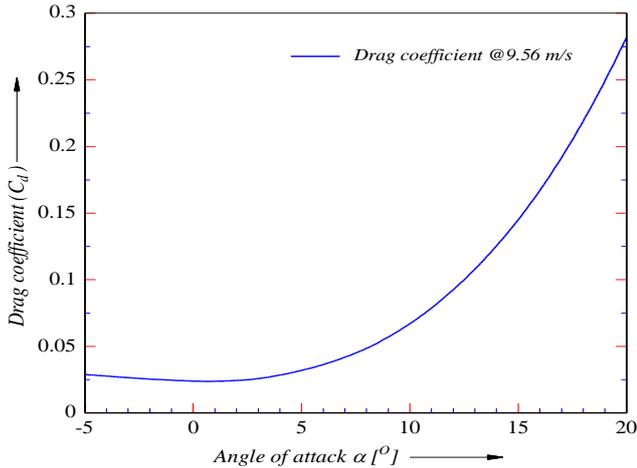
Fig13: CFD result of  $C_d$  vs. AOA for - NACA 63-415 @ 9.56 m/s
