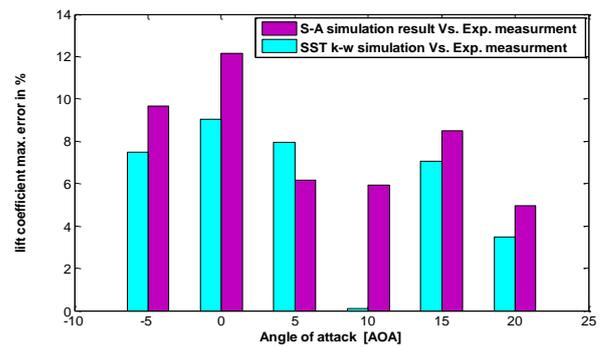
Fig10: S-A and SST  $k-\omega$  model with experimental result max. Error in % for lift
