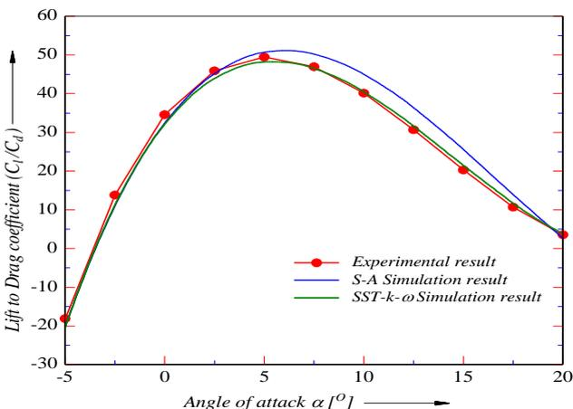
Fig9: Comparison of experimental and CFD result of lift to drag ratio
