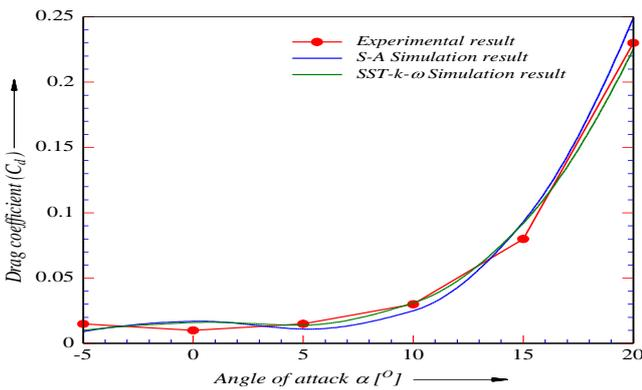
Fig8: Comparison of experimental and computed results for drag coefficient.
