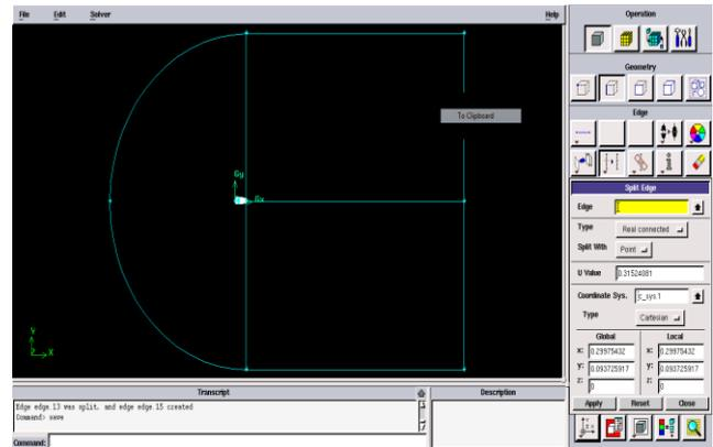
Fig3: Far field boundary and domain developed on GAMBIT
