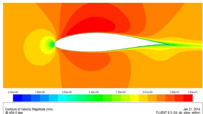
Fig18: Contour of velocity magnitude at  $0^{\circ}$  AOA with the
