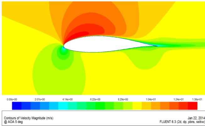
Fig19: Contour of velocity magnitude at 5° AOA with the SST k- $\omega$  turbulence model
