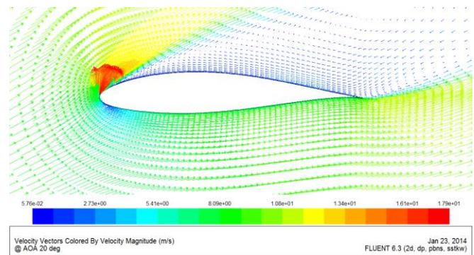
Fig23: Velocity vectors colored by velocity magnitude at 20° AOA with the SST k- $\omega$  model
