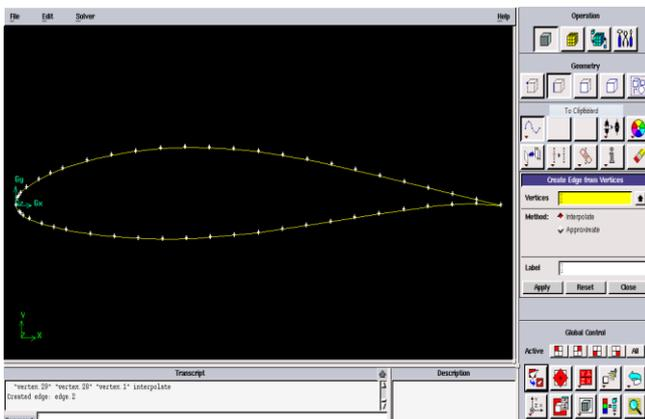
Fig2: NACA 63-415 airfoil geometry developed using GAMBIT
