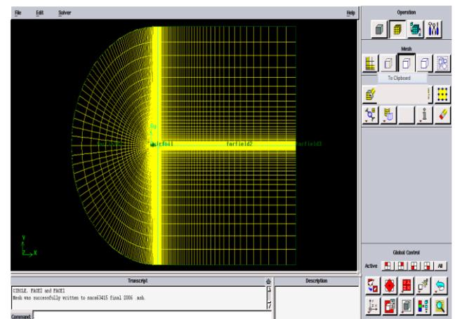
Fig4: Domain meshing over the system using GAMBIT
