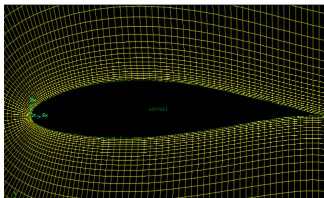
Fig5: Mesh around NACA 63-415 airfoil
