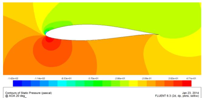
Fig17: Contour of static pressure at  $20^{\circ}$  AOA with the SST k-  $\omega$  turbulence model
