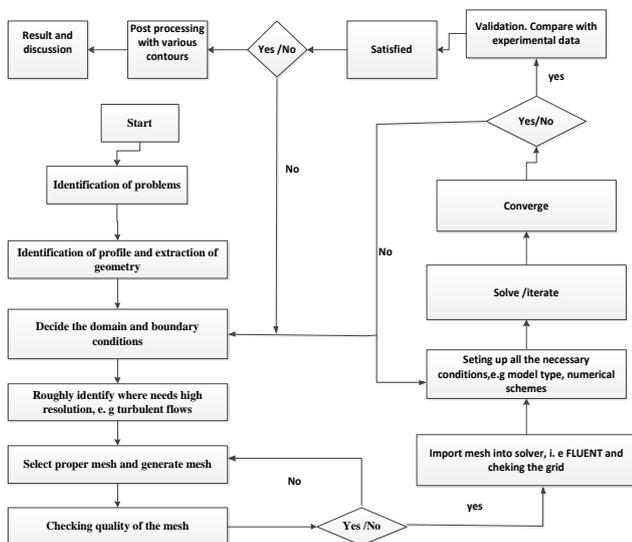
Fig1: Flowchart of typical 2D CFD modeling process
