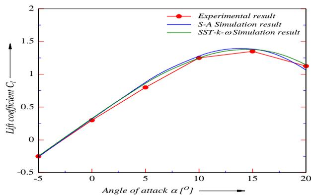
Fig7: Comparison of experimental and computed results for lift coefficient
