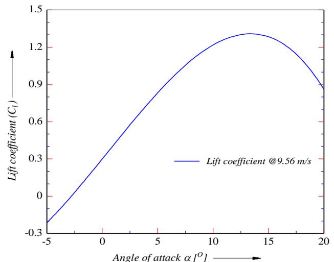
Fig12: CFD result of Cl vs. AOA for - NACA 63-415 @ 9.56 m/s
