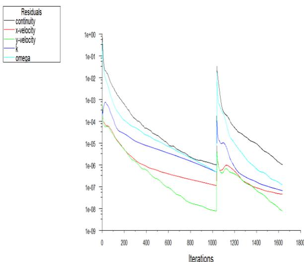
Fig6: Residuals plot with convergence criterion set to  $10^{-6}$
