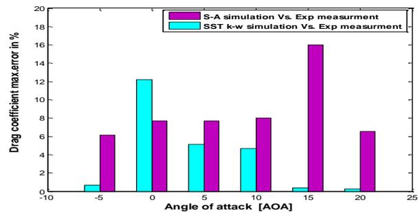
Fig11: S-A and SST  $k-\omega$  model with experimental result max. Error in % for drag
