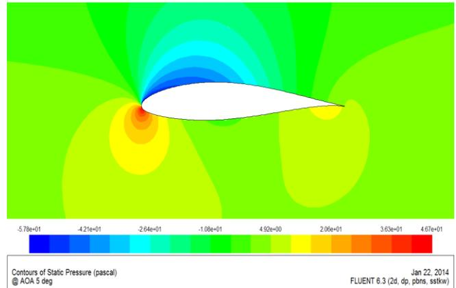
Fig16: Contour of static pressure at  $5^{\circ}$  AOA with the SST k-  $\omega$  turbulence model
