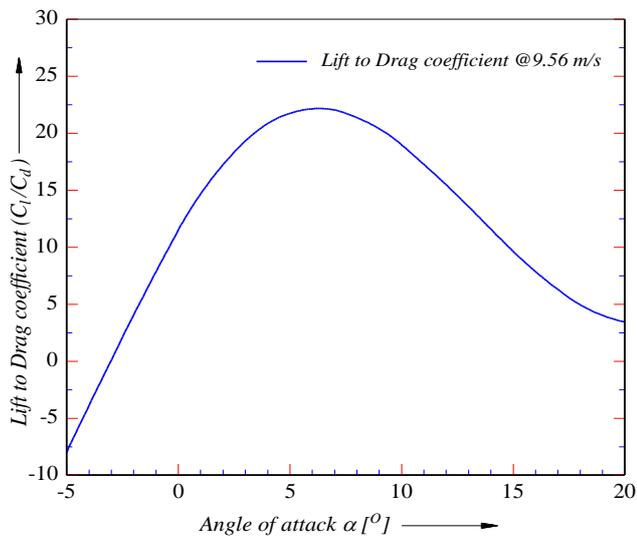
Fig14: CFD result of  $C_l/C_d$  vs. AOA for - NACA 63-415 @ 9.56 m/s
