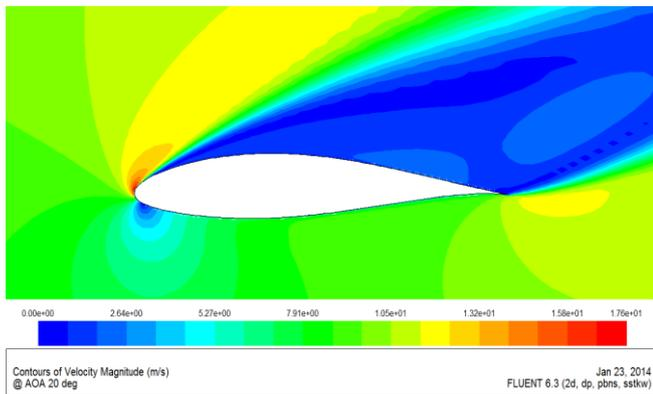
Fig20: Contour of velocity magnitude at 20° AOA with the SST k- $\omega$  turbulence model
