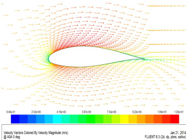
Fig23: Velocity vectors colored by velocity magnitude at 0° AOA with the SST k- $\omega$  model
