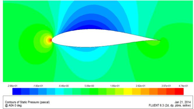
Fig15: Contour plot of static pressure at  $0^{\circ}$  AOA using SST k-  $\omega$  turbulence model
