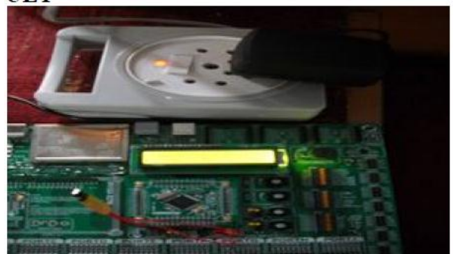
Fig.5. Interfacing of temperature Sensor to Embedded PLC
