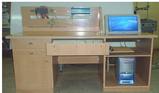
Fig.1. Overview of PLC Workbench
