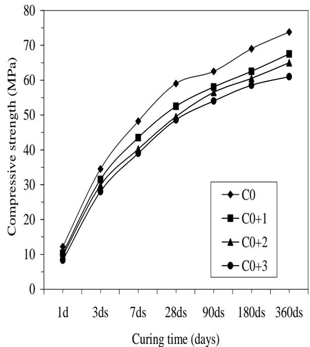
**Fig.2: Effect of Cr (VI) concentration on compressive strength of OPC as a function of curing period**
