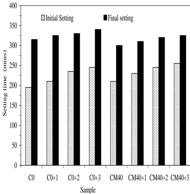
**Fig.1: Setting time of OPC (C0 series) and marble dust blended cement (CM40 series) at various Cr (VI) concentrations**
