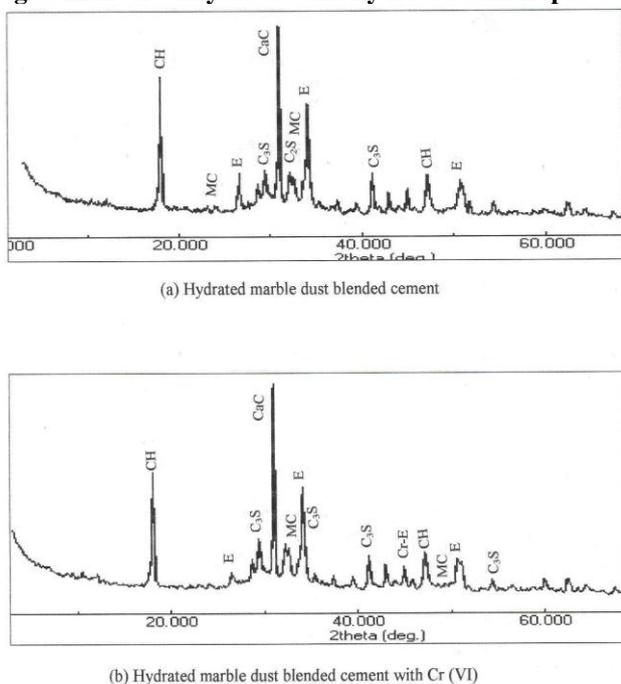
Fig.7: XRD of hydrated marble dust blended cement without and with Cr (VI)
