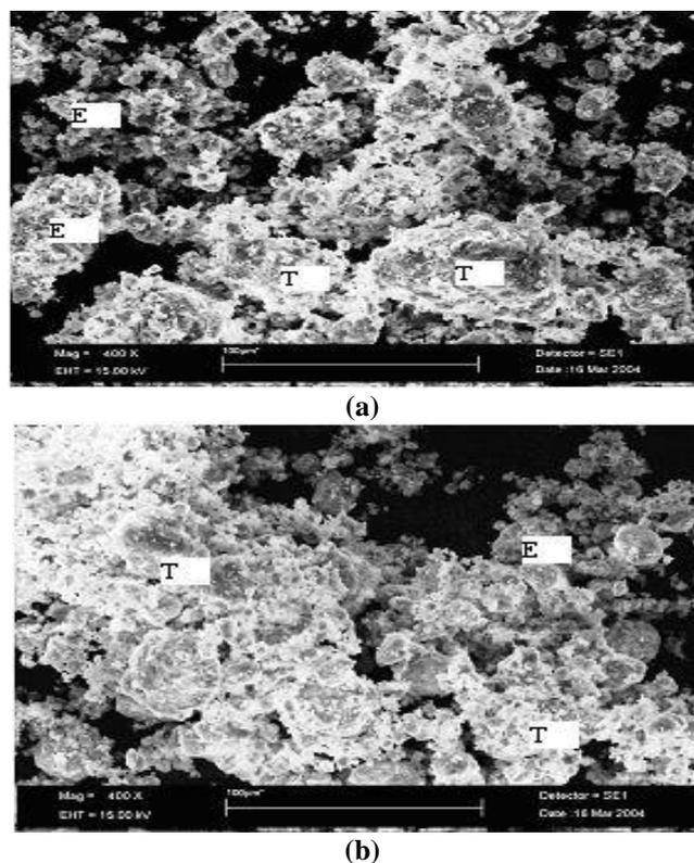
**Fig. 4: SEM of 28 days hydrated OPC without and with Cr (VI) (a) C0 (b) C0+1**
