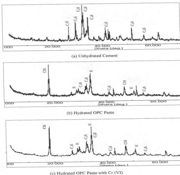
Fig.6: XRD of Unhydrated and hydrated cement paste
