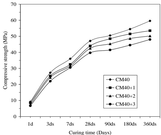
**Fig.3: Effect of Cr (VI) concentration on compressive strength of marble dust blended cement as a function of curing period**
