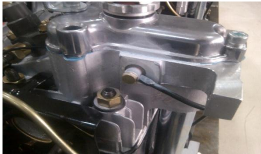
Figure-4 Developer spay use for detect oil wetness
