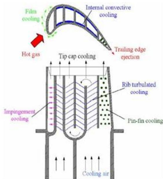
Figure: Cooling types of turbine blade
