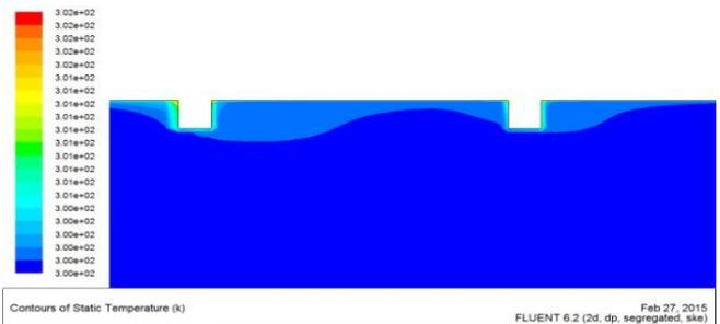
Figure: Temperature change at ribs for Re 20000
