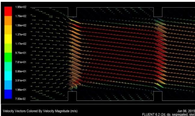
Figure: Velocity vectors between ribs showing turbulence.
