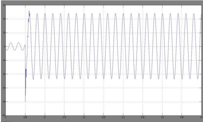
Figure 12: Mitigated current in phase C
