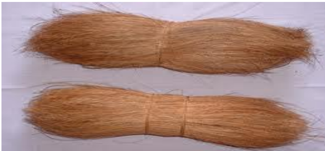
Figure 2: Jute Fiber (D = 2mm, L = 30 mm)
