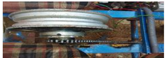
Fig.3.1.1. BLDC motor with chain drive
