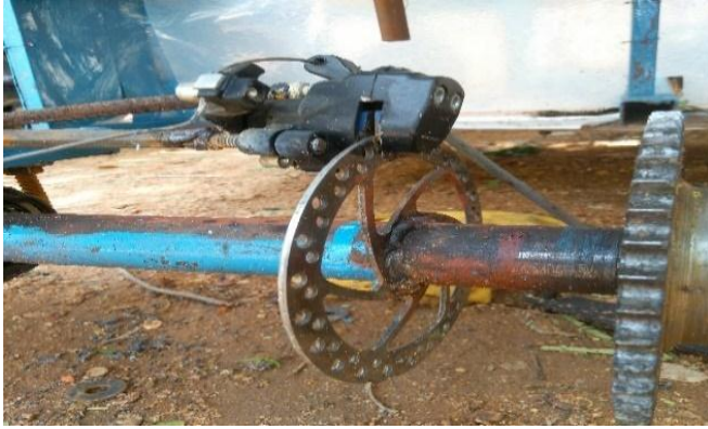
Fig 3.7.1. Experimental braking system used in vehicle
