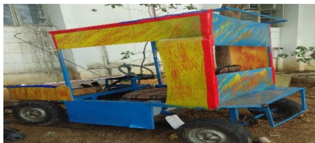
Fig.3.6.1. Body of the solar vehicle according to this report
