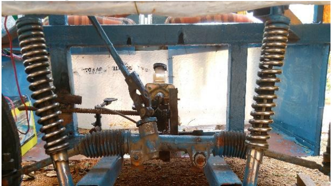
Fig 3.8.1. Rack and pinion steering system
