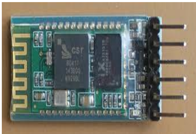
Figure 2 Bluetooth Module- HC05
