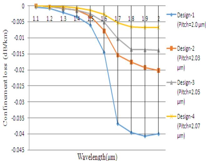
**Fig. 4 Confinement Loss comparison at wavelength 1.55µm between Design-1, Design-2, Design-3 and Design-4 proposed structures**
