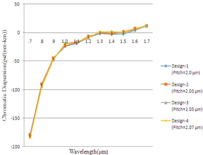
**Fig. 3 Zero order Dispersion comparison at wavelength 1.55µm between Design-1, Design-2, Design-3 and Design-4 proposed structures**
