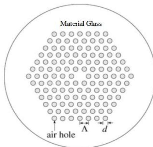
Fig. 1 Schematic representation of a PCF
