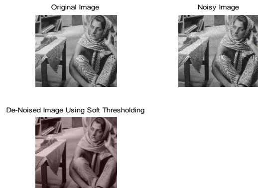
Fig. 2: Original image, noisy image and De-noised image using VisuShrink method for \sigma=15 .
