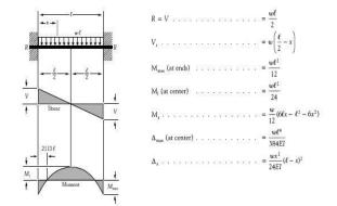
Case 7: Uniformly distributed load over the entire span of continuous with equal distant
