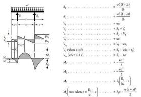
Case 6: Uniformly distributed load over the entire span of both ends fixed
