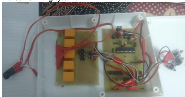
Fig. 9 depicts the actual Circuit i.e. embedded PLC to control the Bottle filling system.
