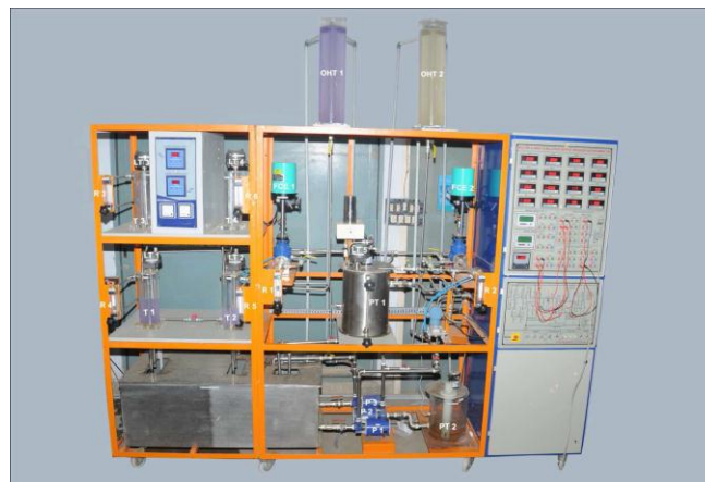
Fig.1. Experimental setup of a two-tank interacting process.
