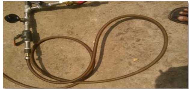
Fig: Air hose Source: photo by author
