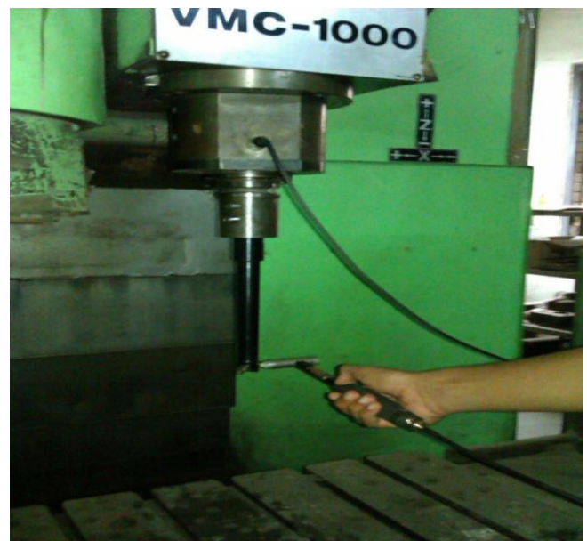
Fig 3: Manual excitation of the bar using modally tuned excitation hammer
