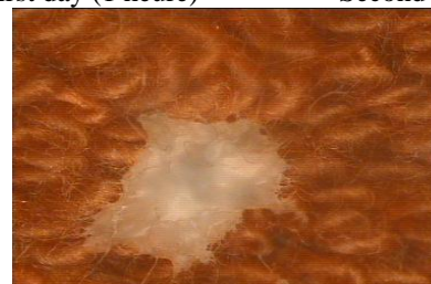
Figure 3: Microscopic visualization of the behavior of a drop of milk on the surface sample
