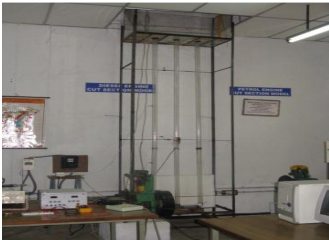
Fig: Fabricated Air Lift Loop
