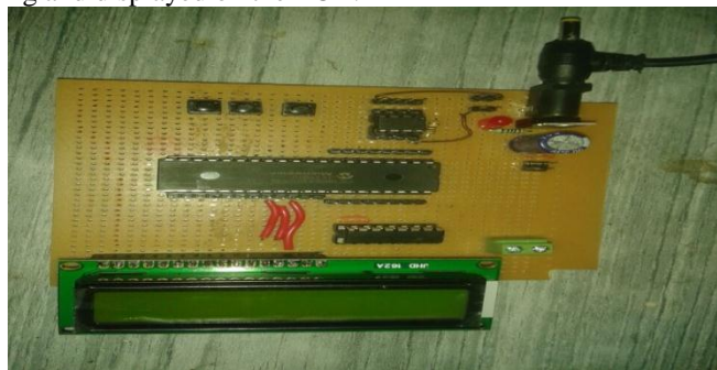
Fig 2: PCB of Microcontroller and Interfacing LOAD CELL:-
