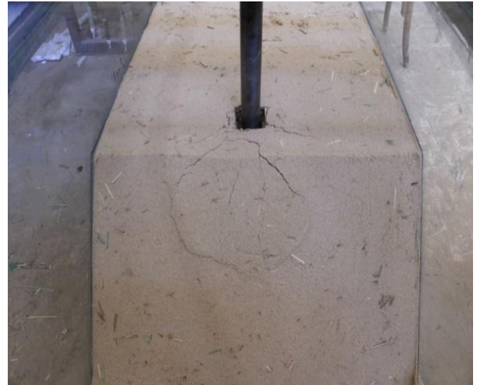
Fig.4 Slope Failure (1H: 1V, R.S = 0.5 % and x = 6 cm)
