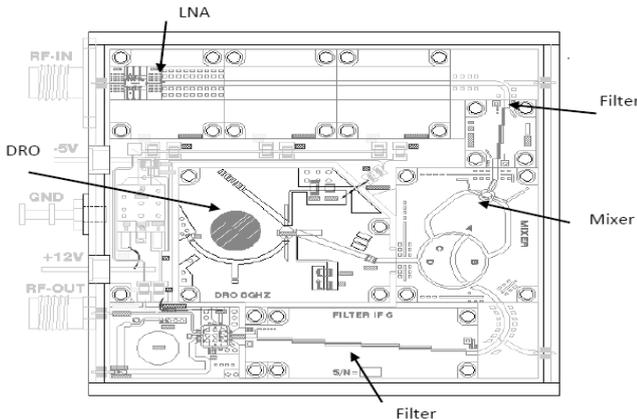
Fig. 2: Layout of the MIC-MMIC Receiving Link
