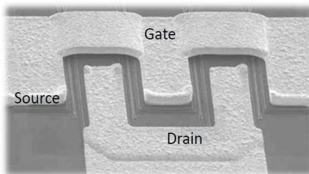
Fig. 6: 0.15 micron PHEMT on GaAs substrate
