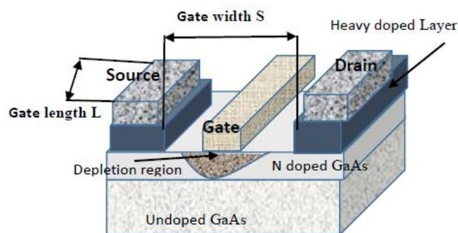
Fig. 7: MESFET cross section on GaAs substrate
