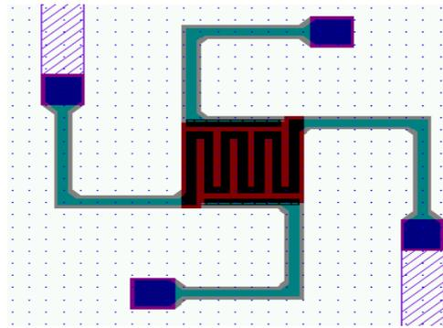
Fig. 19 MEMS Bolometer Layout
