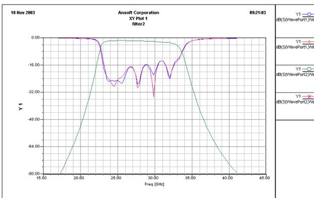
Fig. 22: S Parameters for Filter#2
