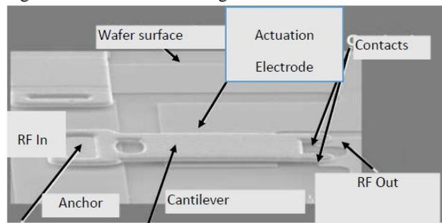
Fig. 15: Surface micromachining
