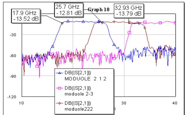
Fig. 26: Switch Filter Bank measured Results unit 1.
