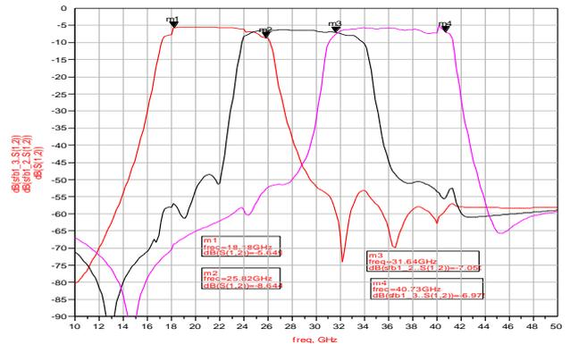
Fig. 25: Filter Bank computed S parameters
