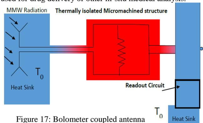
Figure 17: Bolometer coupled antenna
