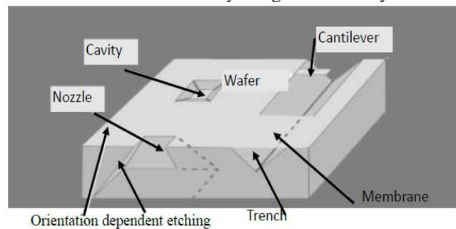
Fig. 14: Bulk micromachining
