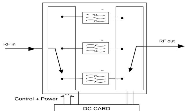
Fig. 20: 18 to 40 GHz Compact Filter Bank Module
