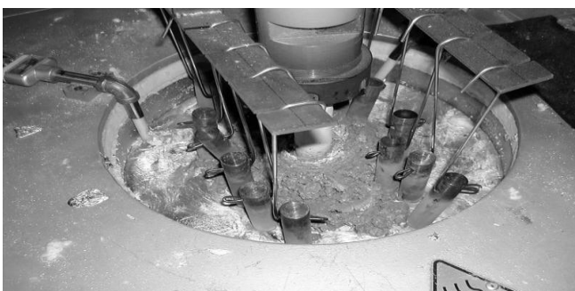
Figure 8. The combined solution to the oxidation problem of the molten zinc corrosion tester
