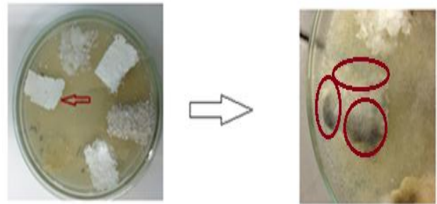
Blend initiated state Blend after 28 days, (heavy growth) Figure.13. Blend (B) biodegradation by contamination
