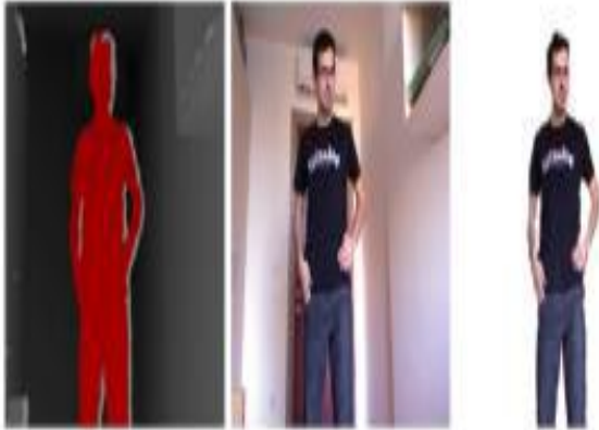
Fig. 7. Background removal. Depth image (left), color image (middle), extracted user image (right)
