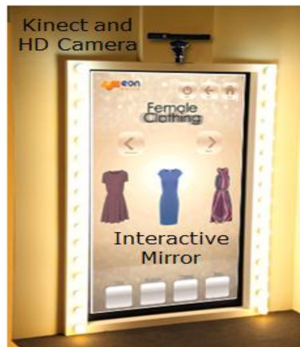
Fig. 1: The front view of the Interactive Mirror with Kinect and HD camera placed on top.
