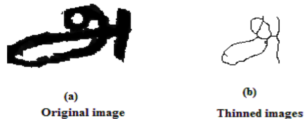
Fig 10 Results of Zhang Suen thinning algorithm applied on character image அ
