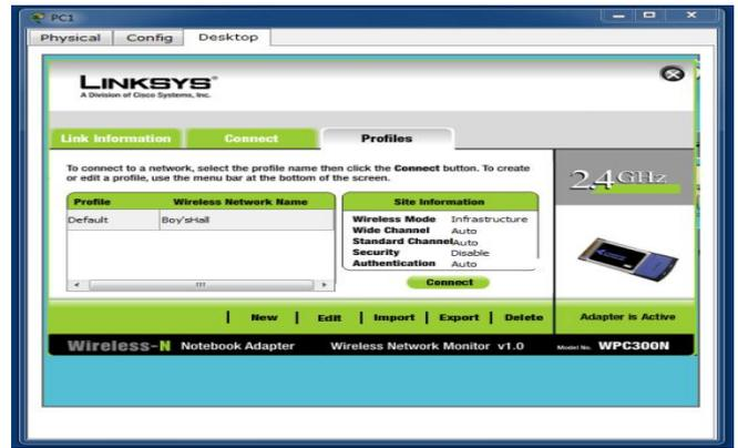
Repeat same procedure to all the devices connected to the Linksys Wireless router R0.
