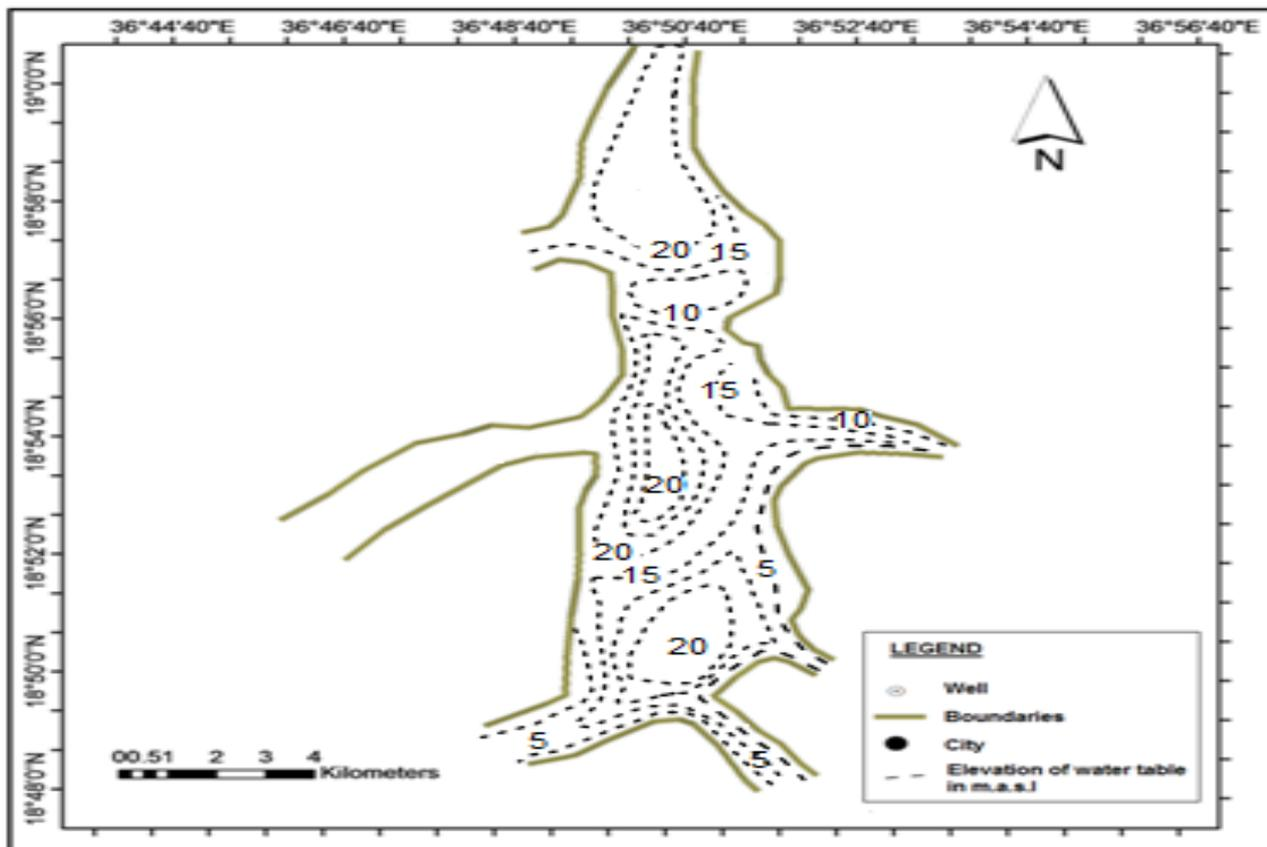
Fig. 6: Aquifer thickness map as determined by VES method.
