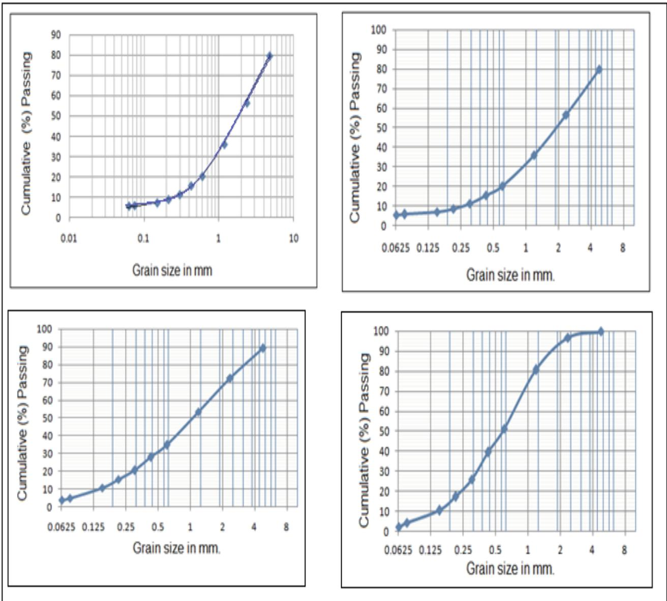
Fig. 8: Samples of grain size distribution curve showing well graded samples.
