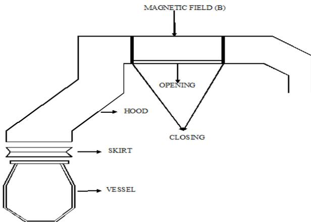
An electromagnetic field will be applied into a portion of horizontal part of the hood as shown in fig. As the off-gases pass through it, it will attract magnetic particles. As major portion (about 40%) of particles are separated here, only those particles, which are non-magnetic, will move forward. Thus rest portion of the cleaning system will come into contact with lesser amount no. of dust particles. Thus it will not require monthly cleaning.
