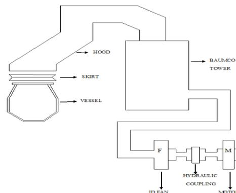
Fig. 1. Schematic view of a gas cleaning system
