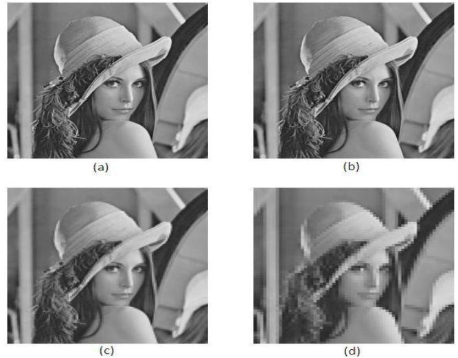
Figure 1 : Lenna image compressed using (a) FELICS (b) JPEG (c) 2-level DWT+FELICS (d) 3-level DWT+FELICS
