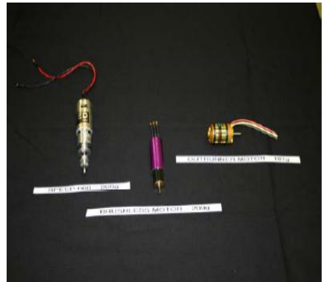
Fig.6. Similar motors using different configuration technologies [10]
