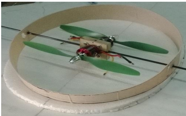
Fig 4:- Cowling with thrust vectoring mechanism
