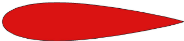
Fig .2. Section of Conventional rudder
