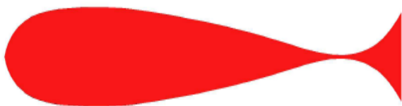
Fig 3. Section of fishtail rudder
