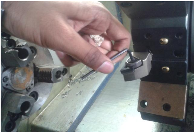
Figure 4: Fitting of insert in the tool holder
