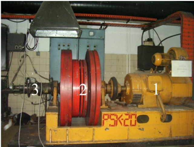
Figure 1. Single-end full-scale inertial dynamometer
