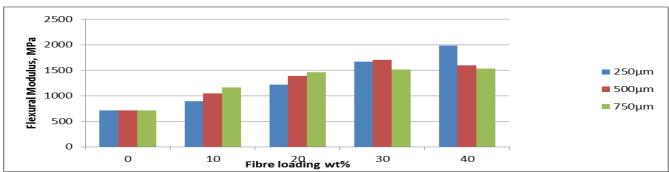
Fig. 2 Flexural modulus of MH-HDPE composites at various fiber loadings and size.
