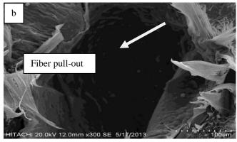
Fig.4 SEM Fractomirographs for Samples with Various Fibers loading; (a)  $10 \% (250 \mu m)$
