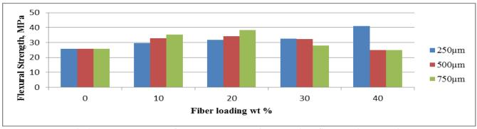
Fig 1. Flexural strength of MH-HDPE composites at various fiber loadings and size.
