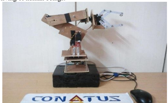
Fig. 8 Final setup of 5 DoF Robotic Arm controlled using PS/2 Mouse
