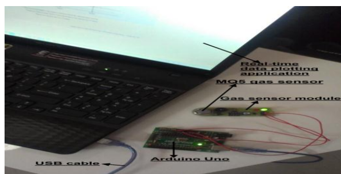
Figure 1. (a) ArduEmission Hardware
