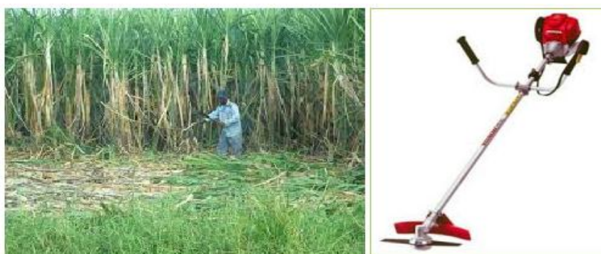
Fig. (13) Illovo brush type cutter with steel knife tested for harvesting sugarcane.
