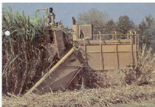
Fig (1) Self propelled whole stalk sugarcane harvester (Louisiana type)
