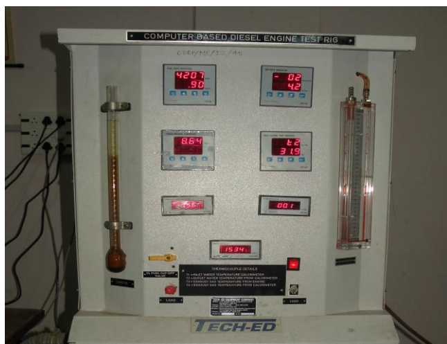
Fig 11 Computerized DA System to check Performance of Engine
