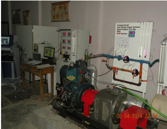
Fig:-1 Experimental set of Cooled EGR
