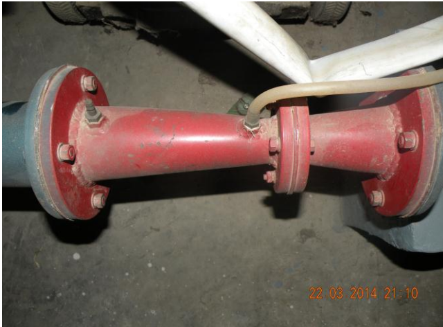
Fig 2. Convergent –Divergent Nozzle
