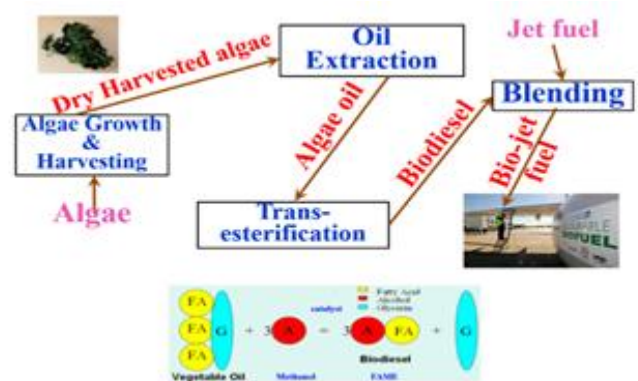
Fig. 2 Steps in the manufacture of Bio-Jet fuel from Microalgae. The transesterification reaction is shown under the transesterification step.
