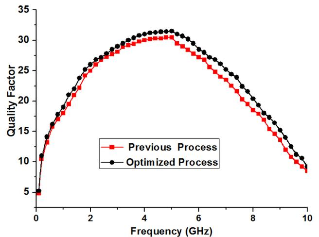
Fig. 7 Fabricated spiral inductor (inner diameter = 150 μm, width = space = 15 μm, turn number = 5, metal thickness = 7.5 μm) measurement result of the Q-factor by both the previous and optimized fabrication processes.
