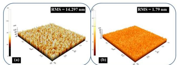
Fig. 6 The three-dimensional (3-D) atomic force microscope (AFM) images of the surface morphology. The images are 3-D AFMs of 10 × 10 μm<sup>2</sup> areas: (a) the previous first metal layer roughness with an RMS value of 14.297 nm and (b) the first metal layer roughness after the optimization process with an RMS value of 1.790 nm.
