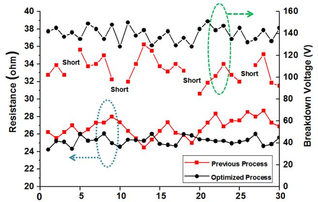
Fig. 5 200 μm × 200 μm TFRs measurement result of resistance and 200 μm × 200 μm MIM capacitors measurement result of breakdown voltage by both the previous and optimized fabrication processes.
