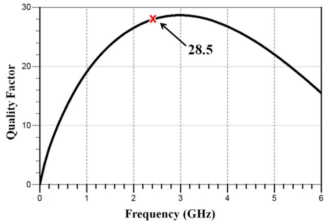
Fig. 3 The quality factor of the designed inductor (L).
