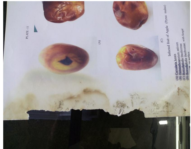
Fig. – 4(A) Glazed paper of a Thesis infested by cellulolytic fungi (from Central Library, DDU Gorakhpur University)
