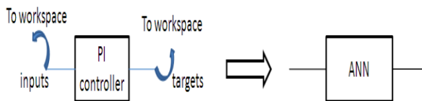
Fig.7: Replacement of PI controller with ANN controller
